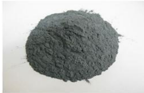
Fig 4.2.2: Silicon carbide 40 \mu size powder
