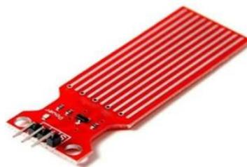
**Figure5. Water Level Sensor**
